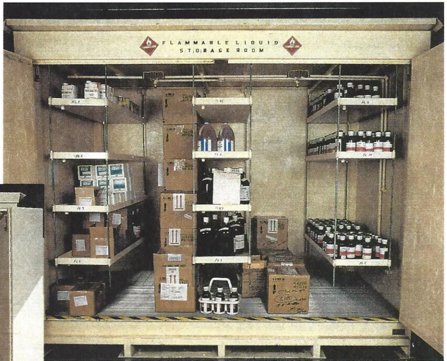
Model #10TDXR. Two door inside seismic storage with secondary containment shelving. Temperature controlled, four hour fire rated and explosion relief.
